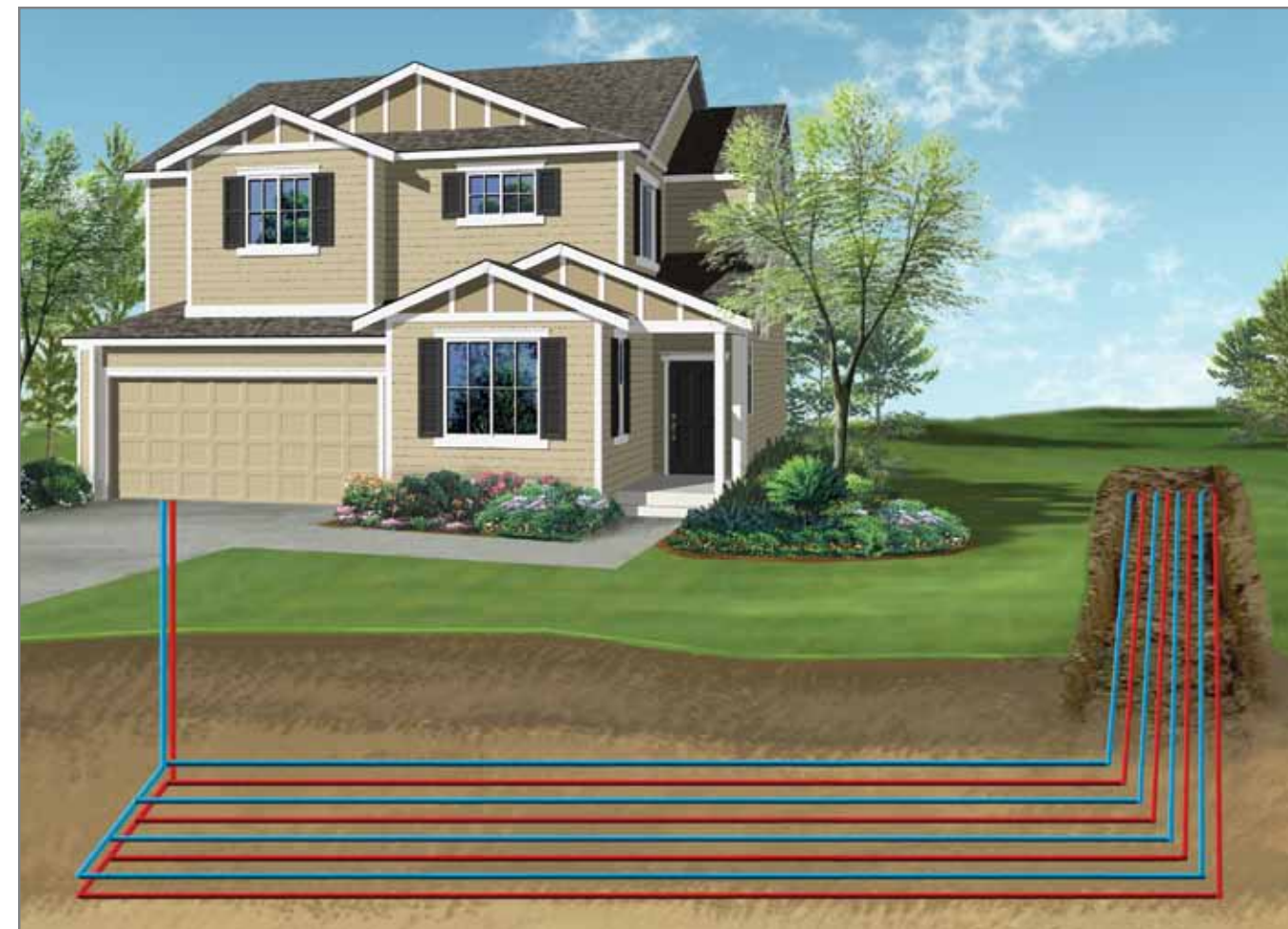
Ground source heat pumps work by taking advantage of the consistent temperature of the ground a few feet below the surface.
