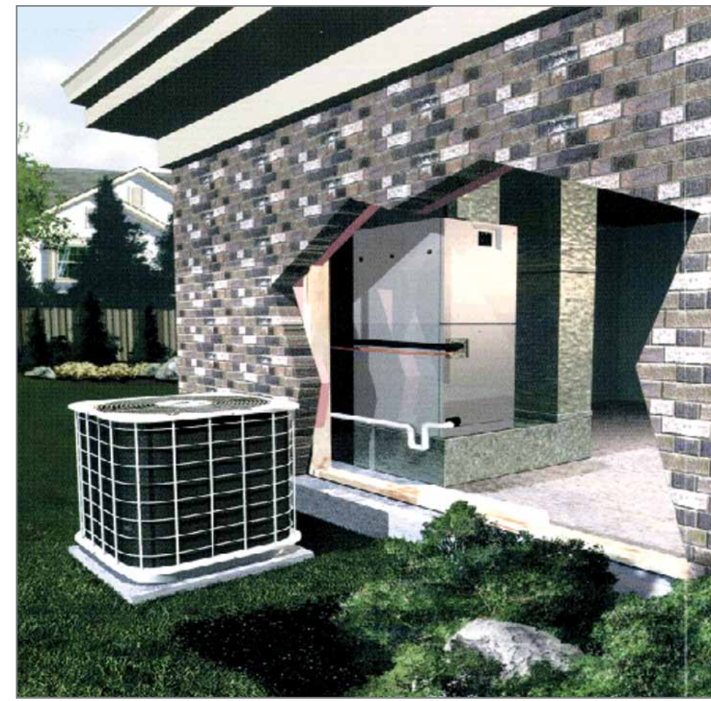
Air source heat pumps regulate the temperature in your home by moving heat from outdoor air into your home. They work best at temperatures above 28° F.
