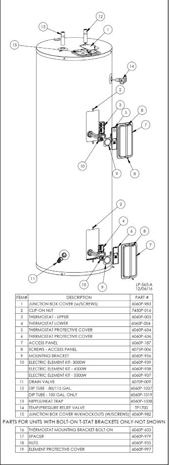
Figure 9 - Replacement Parts - Non-Simultaneous Operation
