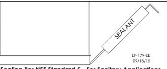
Sealing Per NSF Standard 5 - For Sanitary Applications Apply a 3/8" bead of RTV Silicone completely around the tank to seal the base to the floor and prevent seepage underneath.
