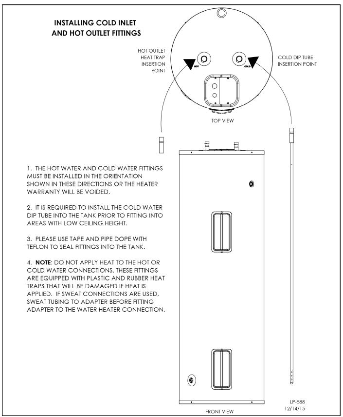
Figure 3 - Installing Cold Inlet and Hot Outlet Fittings
