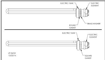
Figure 7 - Heating Element Detail
